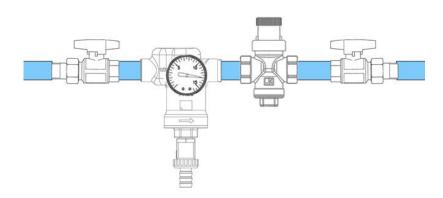
When there is a device which produce or store hot water or pipes are exposed to sudden changes in temperature, an increase of outlet pressure may occur; this event is due to the raise in pressure that follows the temperature rising: an expansion vessel between downstream the pressure reducing valve will avoid this problem.
